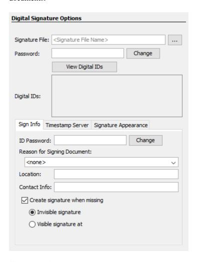
**Signature File** - The full path to the Digital ID file used in the signature on the server. Accepted formats are .p12 & .pfx.
